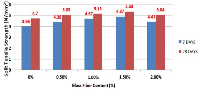
**Chart-6: Split Tensile Strength of M30 Grade Concrete Using Different Percentages of Glass Fibers**
